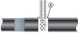
1. For accurate sizing, use a CCG Dimension Tape (A) on the inner and outer cable sheath.
