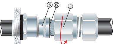
7. Unscrew the body (3). Check that the armour has locked between the cone (5) and cone ring (6). (O-Ring on the cone ring (6) is sacrificial).
