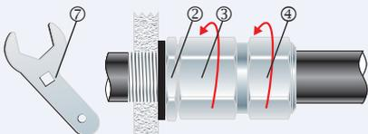
8. Tighten the body (3) onto the inner (2) to the installation torque using a CCG Spanner (7). The Variable Deluge Seal™ will engage automatically as the body is tightened onto the inner (2). Tighten the outer nut (4) to produce a moisture proof seal by turning until the seal makes contact with the outer sheath of cable and then make one full turn.
