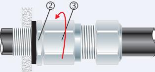
6. Tighten the body (3) onto the inner (2) until hand tight, then tighten with a CCG Spanner (7) with 3/4 turn to lock the armour between the cone (5) and the cone ring (6).
