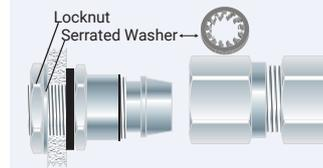
If the apparatus is untapped use a locknut.
