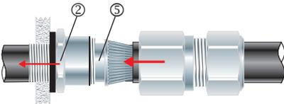
5. Pass the cable end through the inner (2). Splay the armour wires over the cone (5).
