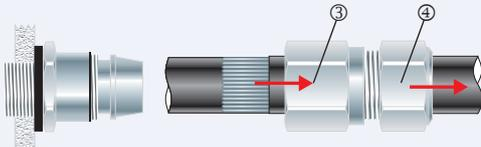
4. Pass the outer nut (4) and the body (3) over the cable.
