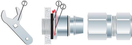
3. To maintain IP66/68 ensure the gasket (1) is in place. Screw the inner (2) into the apparatus. Tighten the inner (2) to the installation torque using a CCG Spanner (7).
