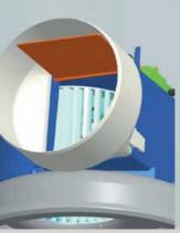
The built-in backdraft shutter is a requirement of building codes and helps achieve 5-Star energy efficiency ratings, but also helps to prevent the entry of insects into the room. This flap opens when the fan is running and closes to prevent backdrafts when the fan stops.
