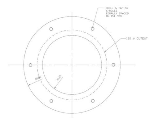
MAT,L 4mm PLATE MS ZINC PLATED SUPPLIED WITH 6 OFF M6 X 30 SET SCREWS ZINC PLATED
