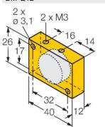
Actuator, rectangular, plastic, attainable switching distance 58 mm on BIM-(E)M12 magnetic field sensors or 49 mm on BIM-EG08 magnetic field sensors; for Q25L linear position sensors: recommended distance between the sensor and magnet: 3...5 mm
