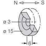
Actuation magnet, Ø 15 mm (Ø 3 mm), h: 6 mm; attainable switching distance 36 mm on BIM-(E)M12 magnetic field sensors or 32 mm on BIM-EG08 magnetic field sensors; for Q25L linear position sensors: recommended distance between the sensor and magnet: 3...4 mm
