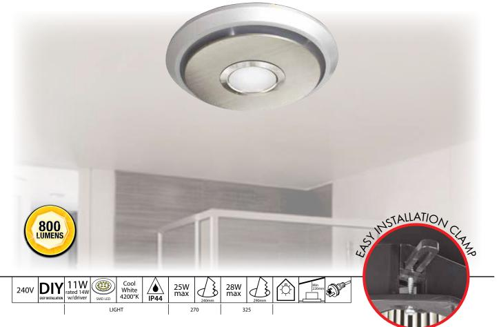
Round design exhaust fan with 800 lumen Umbra-II LED Downlight with a 100 degree beam angle as the centre light source with removable cover with a long life whisper quiet 25W or 28W ball bearing motor. Features easy installation clamps to secure fan into place, a 150mm side exhaust duct to prevent ceiling objects falling through and side damper.
