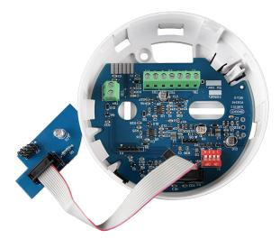
The BAX16 Residential System Interface Base provides the interfacing capability to connect either the EIB650iWX or EIB603CX to the RFS and RFP Residential Fire Systems. The interface base is connected to the respective alarm via a 10-Way ribbon cable which plugs in the connector allocated for the wireless modules in the standard Alarms.
