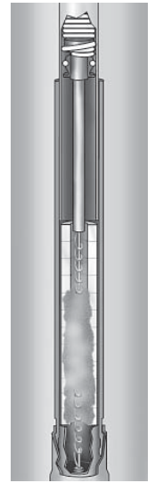
Vapor quenches arc at first current zero
