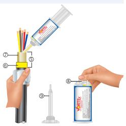
6. Re-insert the barrier pot sub-assembly 5 back into the inner 2.
