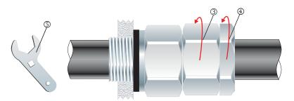
5. Tighten the body ③ to the installation torque using a CCG Spanner ⑤ to produce a seal and grip on the cable. Tighten the outer nut ④ to produce an additional seal and grip on the cable.
