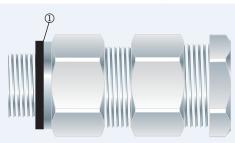
2. To maintain IP66/68, ensure the gasket ① is in place.
