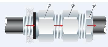
4. Pass the outer nut 4, body 3 and inner 2 (gland assembly) over the cable.
