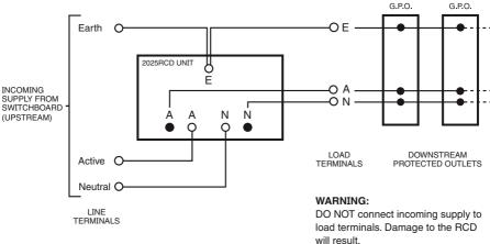
Figure 1. Wiring diagram
