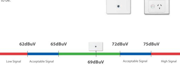
By using the same antenna and 20m of RG6 Quad Shield Coax Cable we can classify the Prime, Fringe and Outer Fringe areas by the level of signal
