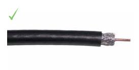
Fold back the first braid then fold back the first foil. Fold back the second braid but DO NOT remove the last foil as this is bonded to the Dielectric. Fold back braid and foil evenly in each direction to ensure the connector slides on easily. A good preparation should look like the following diagram.
