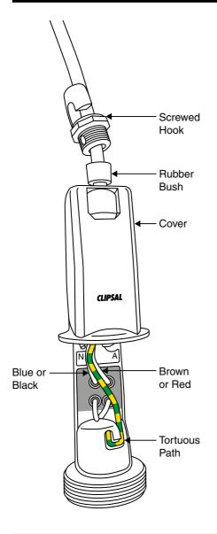
NOTE: Earth wire is connected directly to the socket and Active/Neutral are connected directly to the switch.
