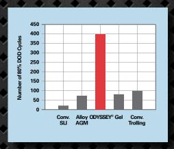
**Long Cycle Life**ODYSSEY® Extreme Series™ batteries routinely deliver up to 400 deep cycle (80%) discharges.
