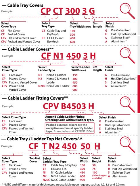
^^MTO and different material thicknesses are available upon request, such as 1.2, 1.6 and 2.0mm. "Please note that the process of Hot Dip Galvanising sheet metal products is not recommended and product distortion is likely to occur as a result.
