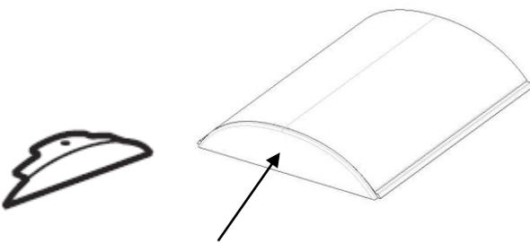
For blanking the end of the floor duct, Cat. No. 032800
