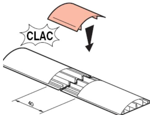
For mounting with floor ducts 92x20mm
