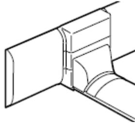
For branching from skirting-trunking 80/120x20 mm to floor duct Cat. No. 032800
