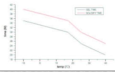
Table 1. shows gel time and complete solidifying time (shown in minutes) curves for installation reference at variable temperatures.
