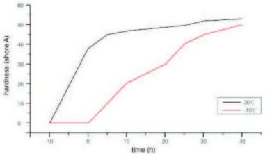
**Table 2**. shows hardness levels (shore A) together with elapsed time in hours at variable temperatures.
