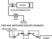
ONE WAY DIMMING (ON/OFF ENABLED)
