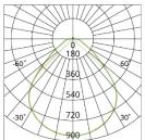
Unit: cd – C0/180 92.0deg – C90/270 91.4deg Photometric diagram shown is for 4500K output.
