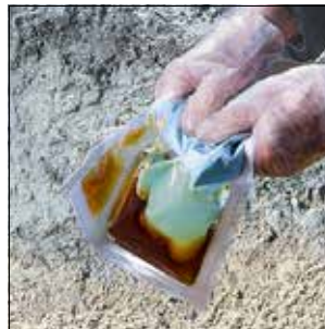
The middle cold seal between the resin and harder component opens by means of pressure.
