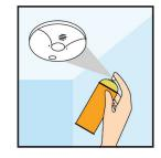
Spray to smoke alarm for 1-2 seconds from a distance of 1-2 metres, alarm will activate within 10 secs if operating properly
