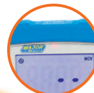
Red Light Indicates detection of Non-Contact Voltage (NCV)
