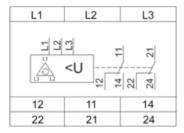
L1,L2,L3 : Supply to be monitored 11-14,12 : 1st C/O contact of output relay
