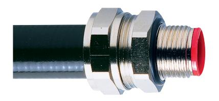
Straight fitting with fixed external male thread. For insertion into threaded entries or knockouts using a locknut to secure.
