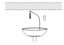
Secure the safety wire using the designated screw point on the hang bracket or other secure point such as ceiling joist.
