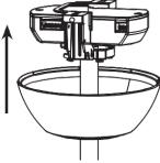
Ensure all wires are tucked neatly into canopy taking care not to cause damage.
