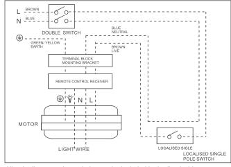
All pole disconnection switch must be included in the fixed wiring.
